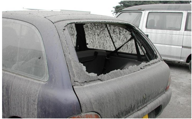
6.噴石よる被害 Damage caused by cinders
